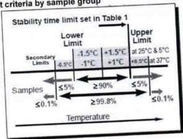
Allowable range of end points: Table 4 defines the allowable range of end points such that 90% of a production lot must reach the end point at the specified time within a range of ±1°C and that 99.8% of the lot must reach/end point within a range of ±1.5°C.
